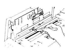
Wipe the white plate with the cleaning pen. S. Document Feed and Pick-up Rollers Wipe the document feed and pick-up rollers with the damp cloth while rotating them. Note: Be careful not to damage the S1
